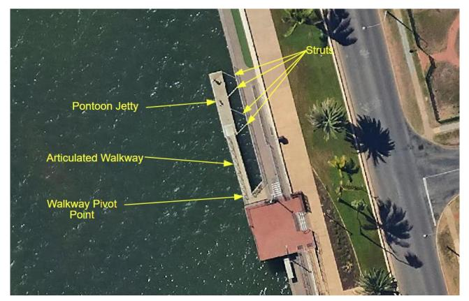
The pontoon jetty struts were removed temporarily during recent capping beam works to provide access for contractors completing that capping beam work. Upon removal it was found that almost every strut had defects ranging from:
