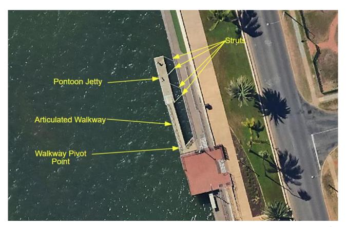
The pontoon jetty struts were removed temporarily during recent capping beam works to provide access for contractors completing that capping beam work. Upon removal it was found that almost every strut had defects ranging from:
